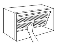
4. Loosen screws in the rear grille to about 1/8". Then, while holding on to the wire loop, tip the grille and pass it through the rear opening of the sleeve. The baffle contact area should be on the left.
